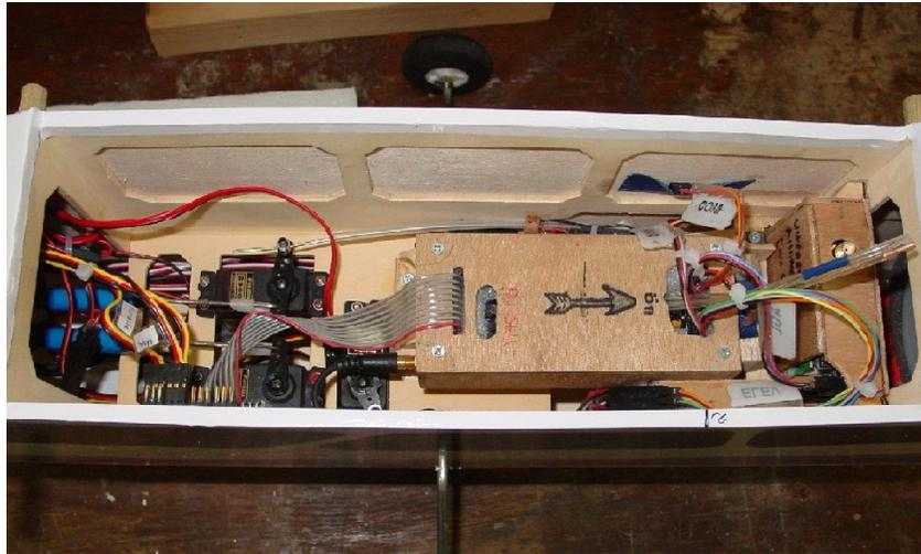
A box was made for the autopilot and the AGL sensor circuits from wood and foam rubber to guarantee the security of them in the occurrence of an accident. Substitutes for the possible breakable parts of the aircraft were made, and were used incidently.
