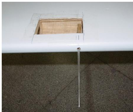
A pitot static tube was made using two different diametered metal tubes. Four wholes that make 90 degrees with eachother were made on the wider tube. These wholes were located  $8 \times \text{diameter length (3mm)} = 2.4\text{cm}$  away from one of its open
