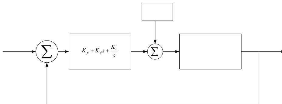
Figure 5.4: Representation of PID control feedback loop
