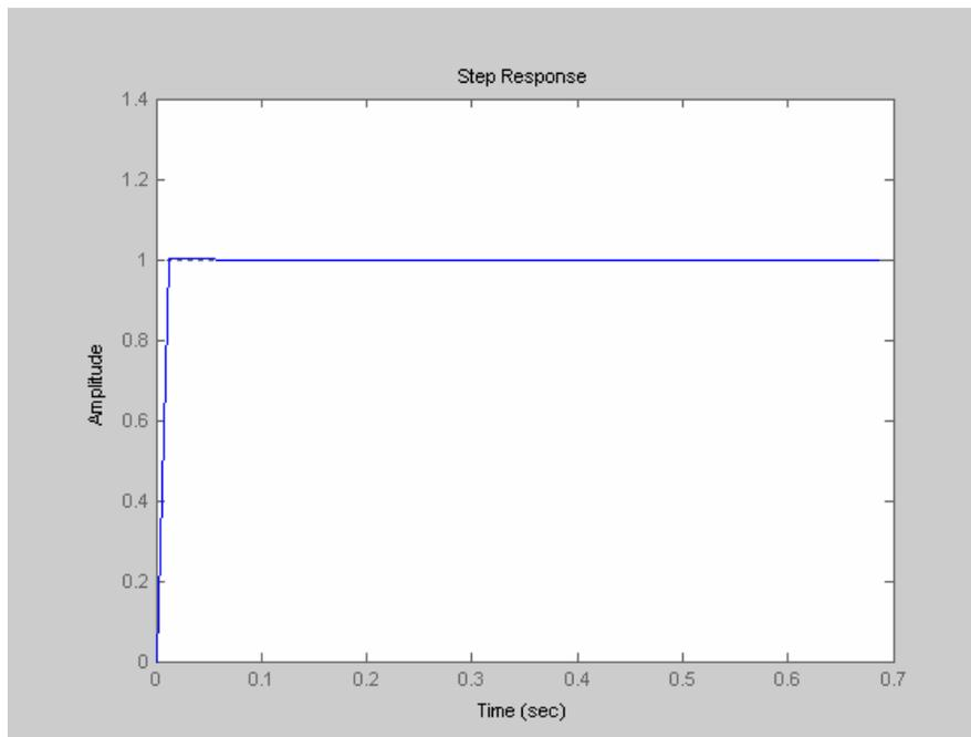
Figure 5.5: Closed loop Transfer Function for elevator from pitch transfer function for level flight
