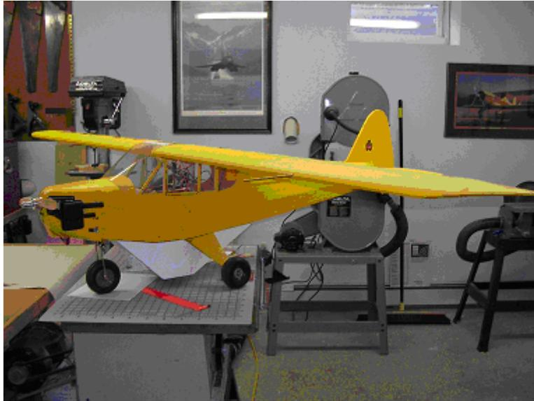
Figure 1. PolyUAV: Instrumented ¼ scale J3 Piper cub
