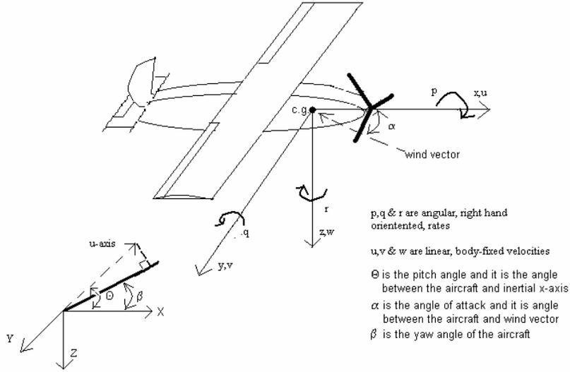
Figure 5.1: Body Fixed Coordinate System Description
