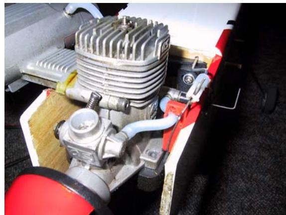
**Figure 10-** An engine cutoff switch is mounted to kill the engine in the event of a systems failure.
