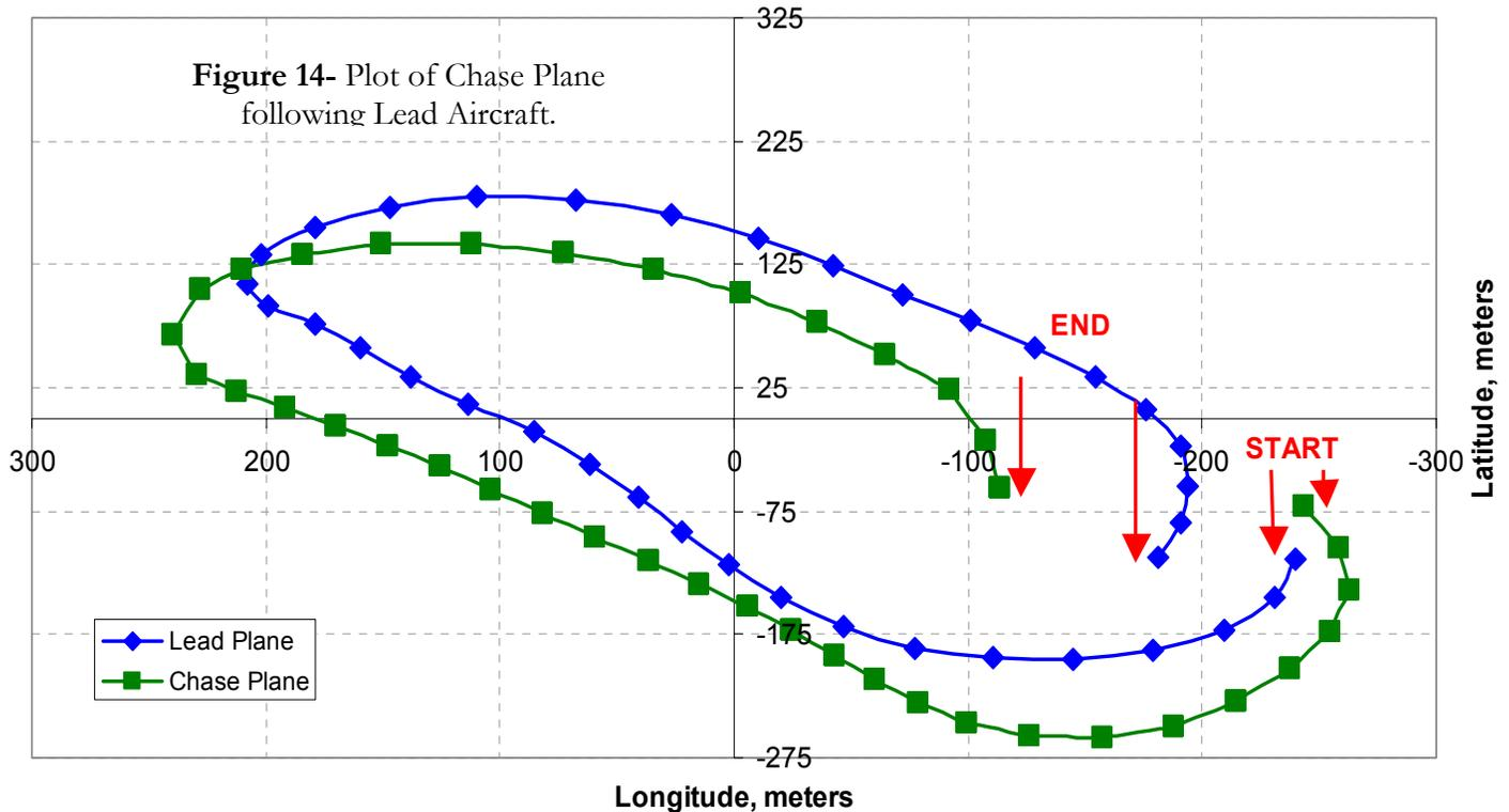
**Figure 14-** Plot of Chase Plane following Lead Aircraft.
