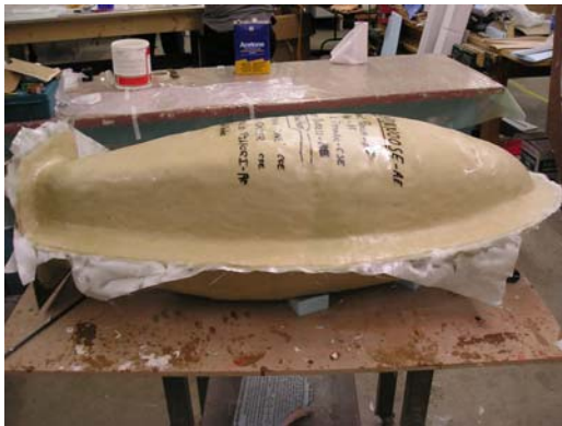
Figure 10: Final Sealing of Mold
