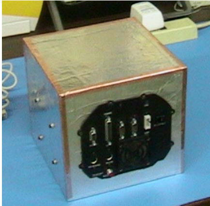
Figure 18: RF Shielded Enclosure
