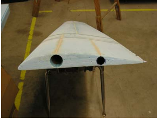
Figure 2: Carbon Tube Installation
