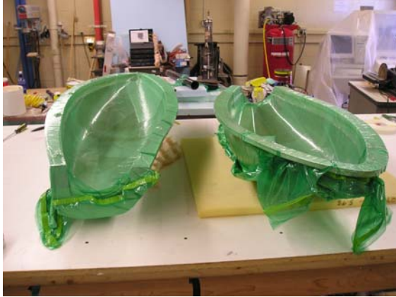
Figure 12: Vacuum Bagged Molds
