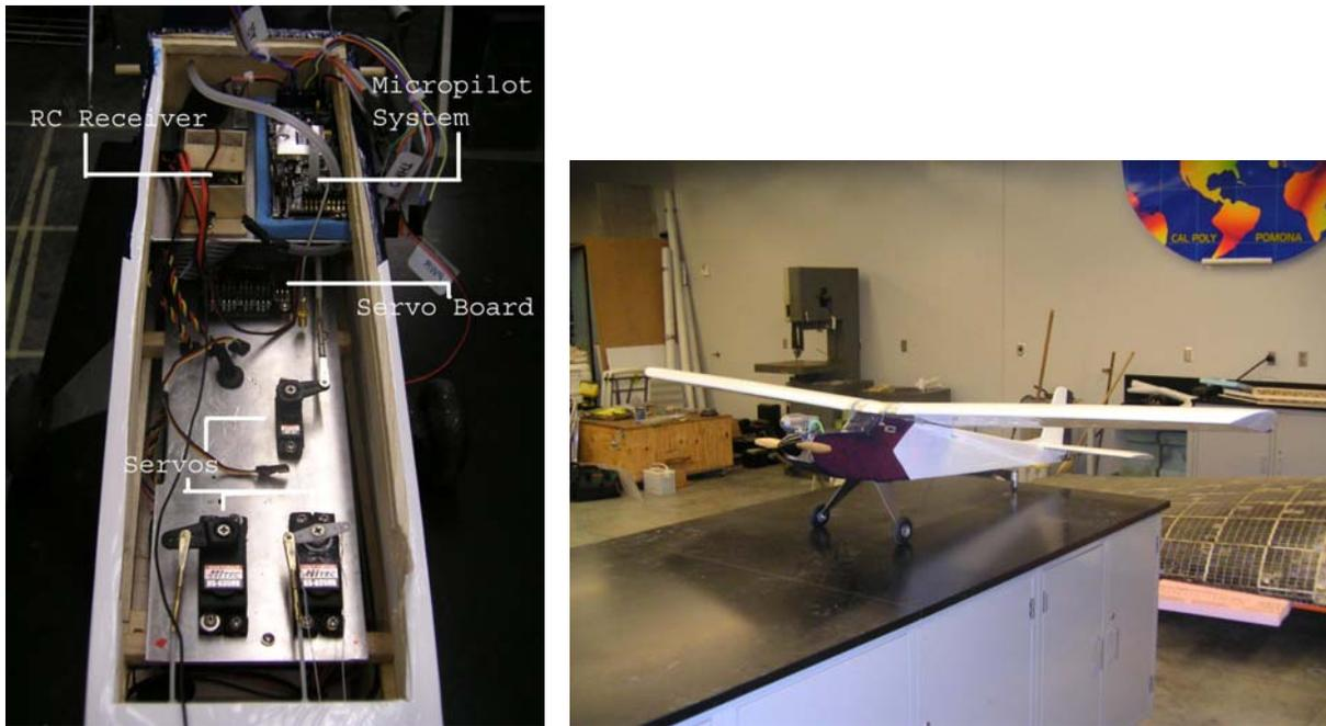
**Figure 1. Detailed View of ARIES Flight System**
