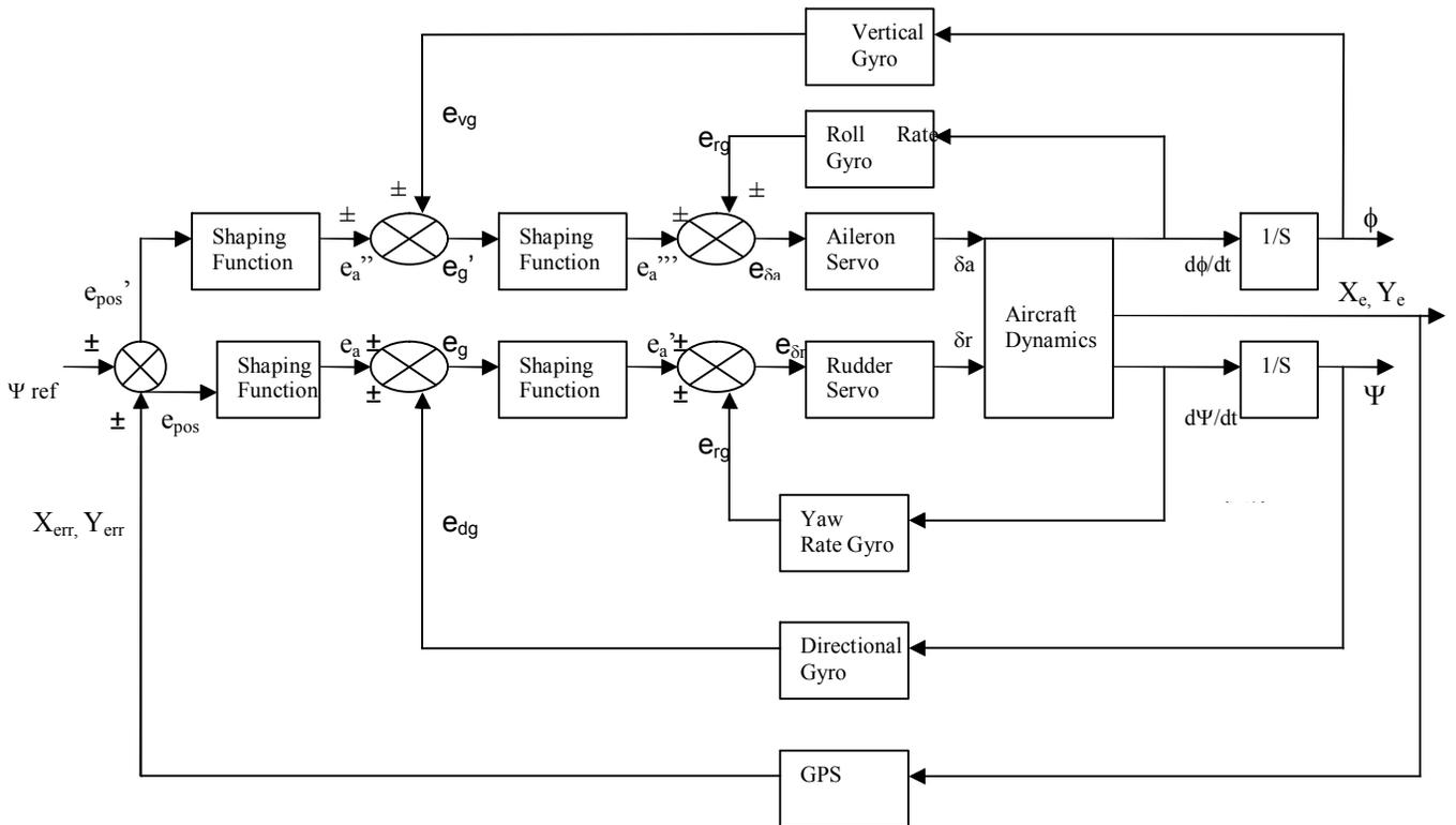
**Figure 3. Lateral Cruise Control Loop**
