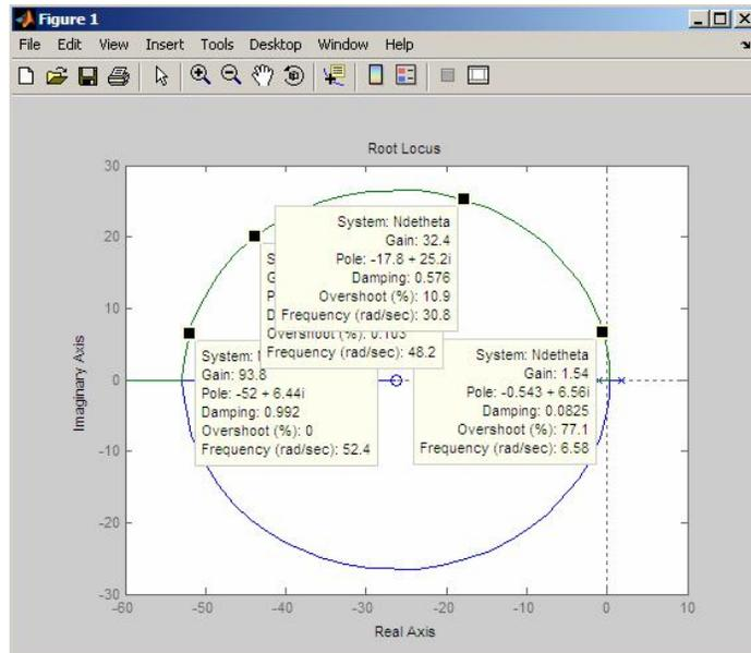
**Figure 4. Open Loop Root Locus Plot for Initial Aircraft Directional Response Due to Elevator Deflection**
