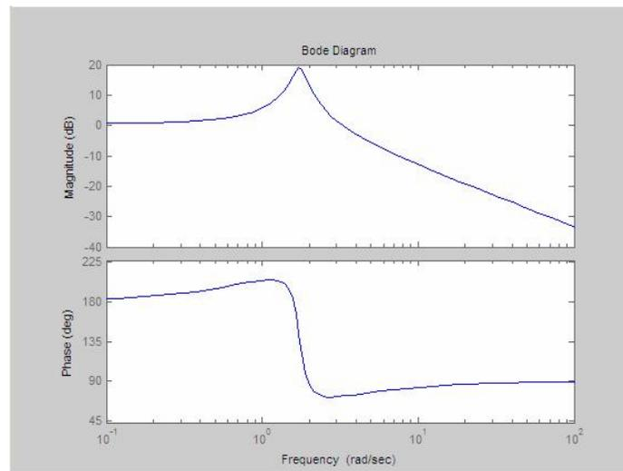
**Figure 5. Bode Plot for Initial Aircraft Roll Response Due to Elevator Deflection**
