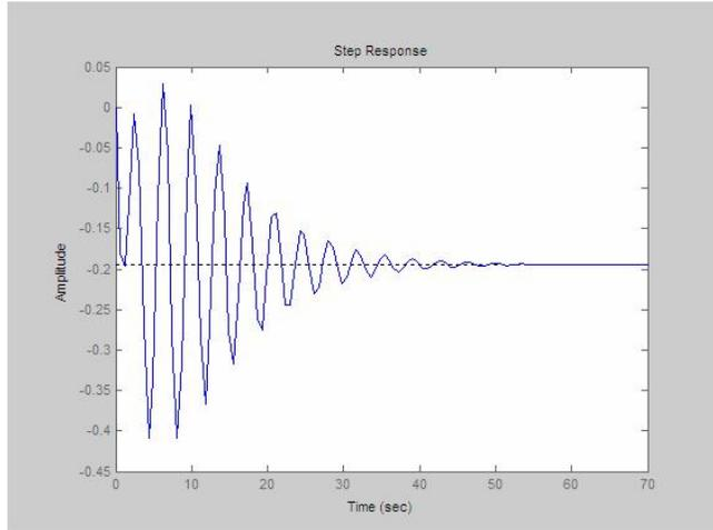
**Figure 6. Step Response for Initial Closed Loop Aircraft Response for Roll due to Aileron Deflection**
