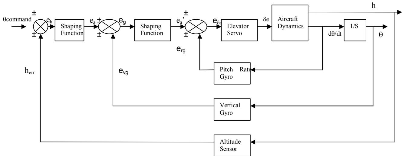
**Figure 2. Longitudinal Cruise Control Loop**
