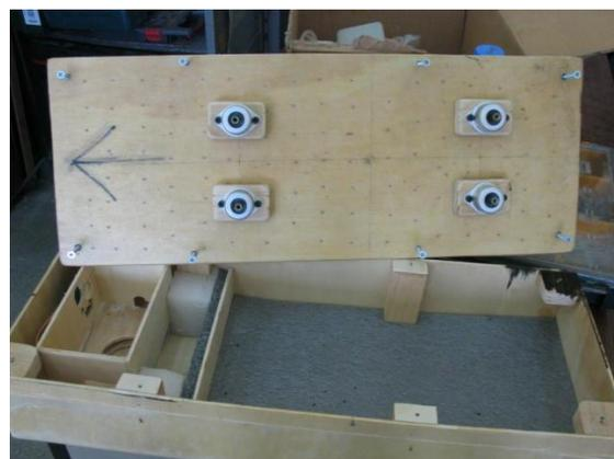
Then this box is mounted by vibration emitting nuts and bolts to the helicopter. To fit this box under the helicopter new landing gears were made from glass fiber and epoxy.
