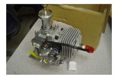
Thus a second, larger engine replaced the Zenoah to deliver this power. A 39.4cc Brison engine was installed that not only weighed approximately the same as the
