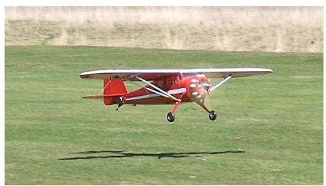
The model aircraft has a 98 inch wingspan with a wide chord giving it the capability for lifting large loads. With so much wing area, the wing loading is low allowing for low speed landings. It also offers an interior with enough volume for a sizeable payload. With such a large aircraft, there would be no problems in carrying all the present and future avionics and camera equipment. A high winged aircraft, the Monocoupe is also inherently stable.
