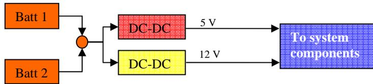
**Figure 7:** Basic Power schematic showing power redundancy to the FC
