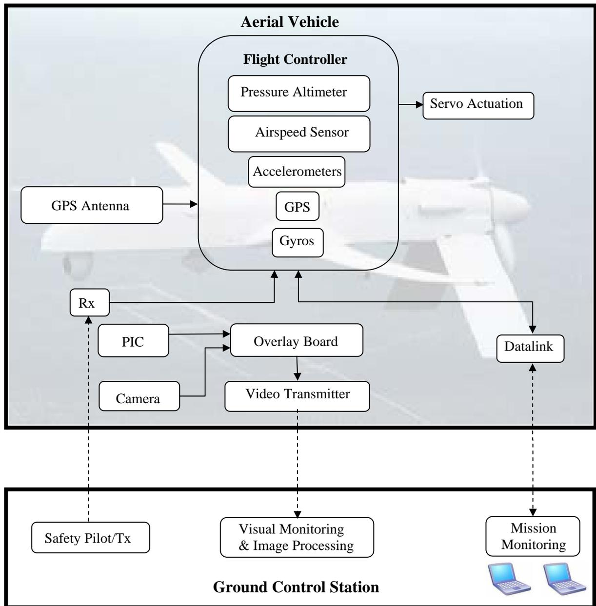
**Figure 2:** System Architecture
