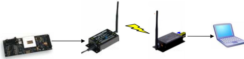
**Figure 5:** Flow diagram of wireless communications from XAVIER to the GCS
