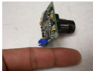
Figure 7: The EverFocus CCD Camera
