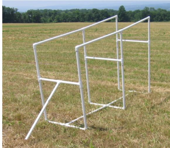
Figure 4: Fully Assembled Launcher
