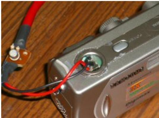
A small electronic board is placed between the camera's button and the parallel port of the flight computer so that the camera can be controlled from the image processing program. When the program detects an object it takes a photo with this camera automatically.
