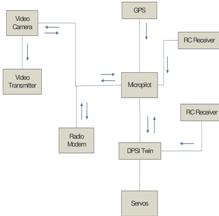
Figure 3.1: X<sup>2</sup>ipiter UAV System
