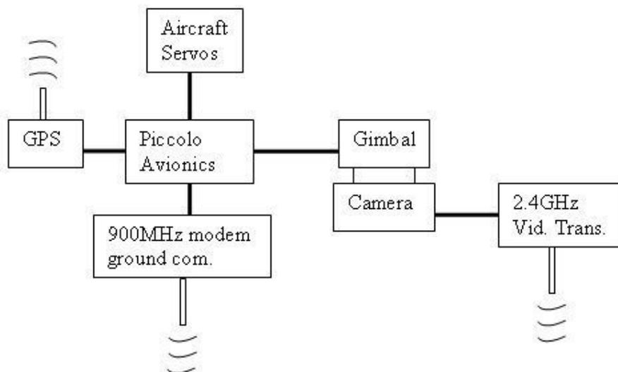
Figure 2: Block Diagram of Subsystems Onboard Athena
