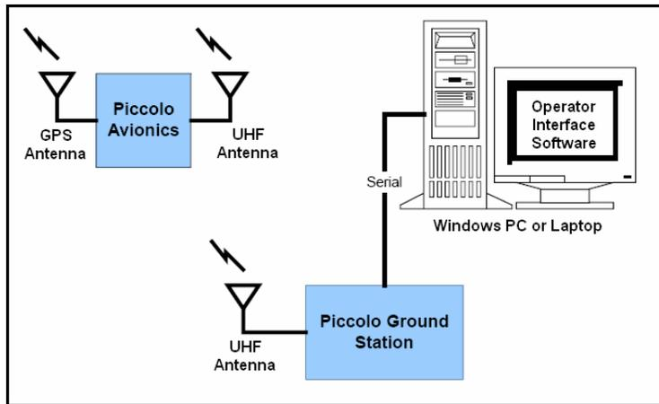
**Figure 5 - Piccolo Block Diagram**
