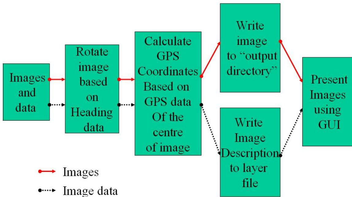
**Figure 10 – Camera Stitching System Block Diagram**
