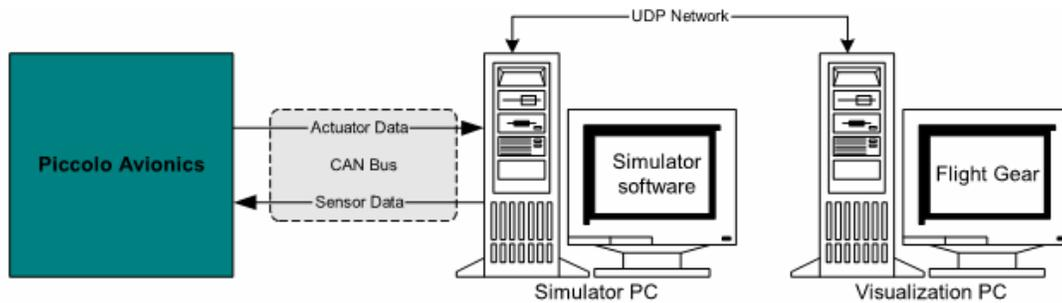
**Figure 12 – Hardware in the loop simulation<sup>3</sup>**
