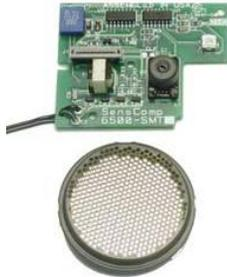
**Figure 2: AGL Board and Transducer**
