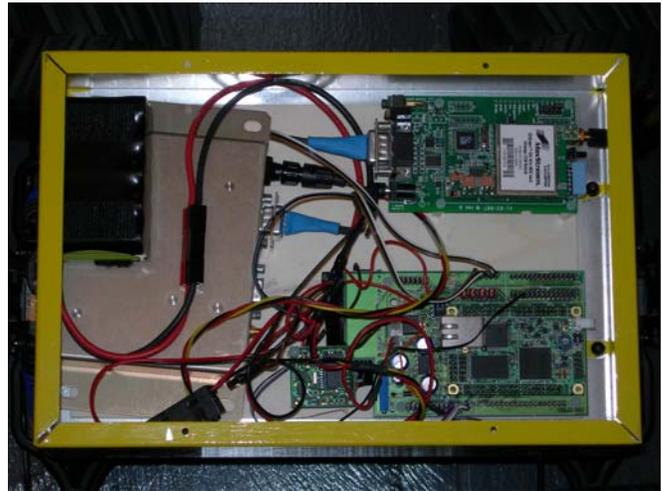
Figure 5: UGV Vehicle Control System, w/ Trimble GPS, Maxstream Modem and Suzaku visible
