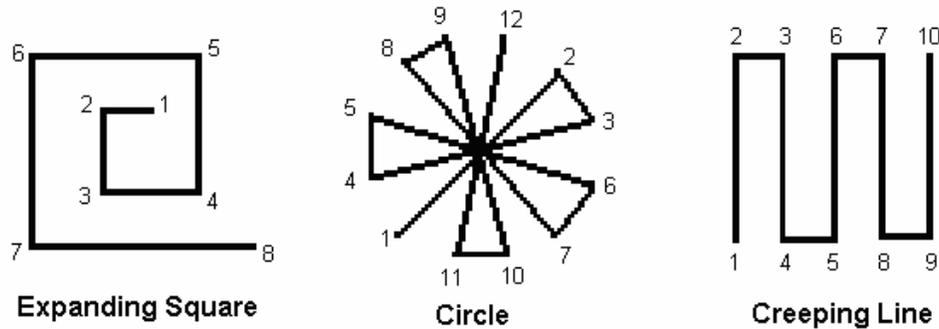
**Figure 9.** Traditional search-and-rescue mission flight patterns used for missing persons searches. [Coast Guard Boat Crew Seamanship Manual. 27 Feb 1998]
