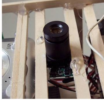
**Figure 6.** Black Widow AV KX141 High Resolution Color CCD Camera
