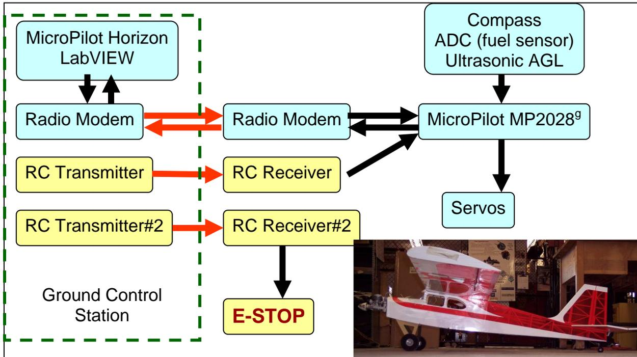
Figure 5. Diagram of autopilot data and control.
