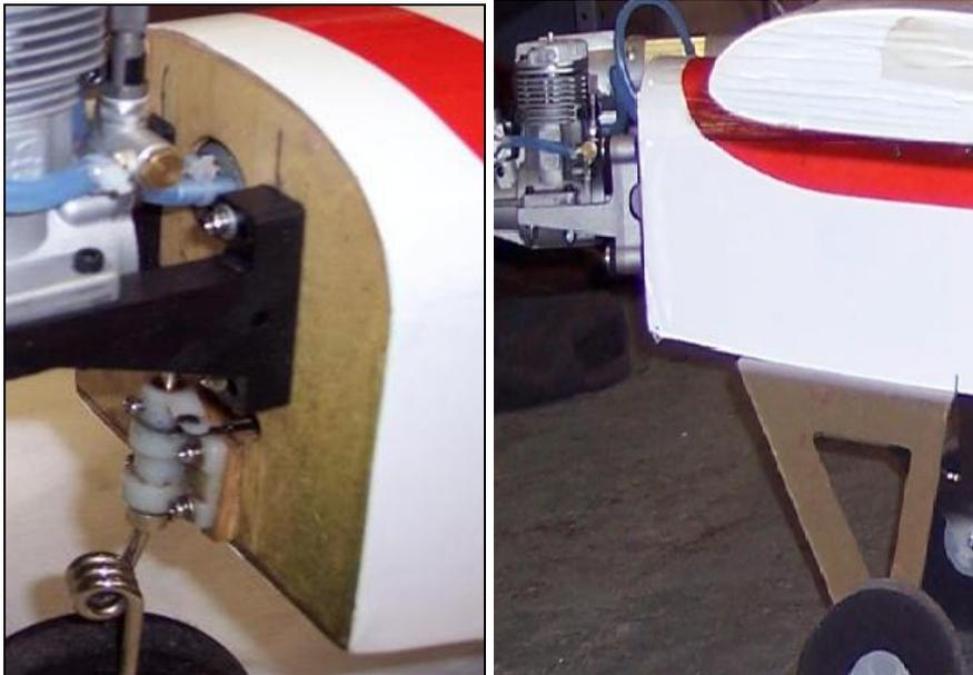
Figure 1. The firewall and original landing gear(left), the new tail dragger gear(right)
