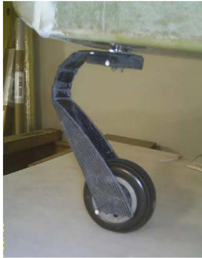
**Figure 9 Nose Gear of X<sup>2.5</sup>**
