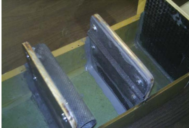
**Figure7 Wing-Fuselage Attachment**
