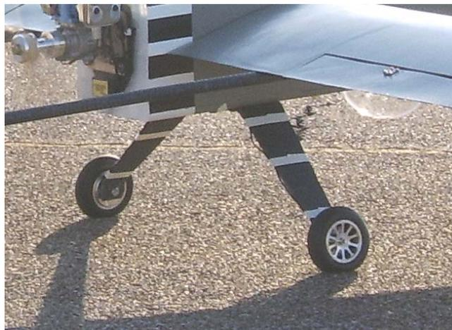
**Figure 10 Main Landing Gear of X<sup>2.5</sup>**
