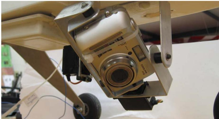
**Figure 5: Nikon P2 in two-axis camera mount**
