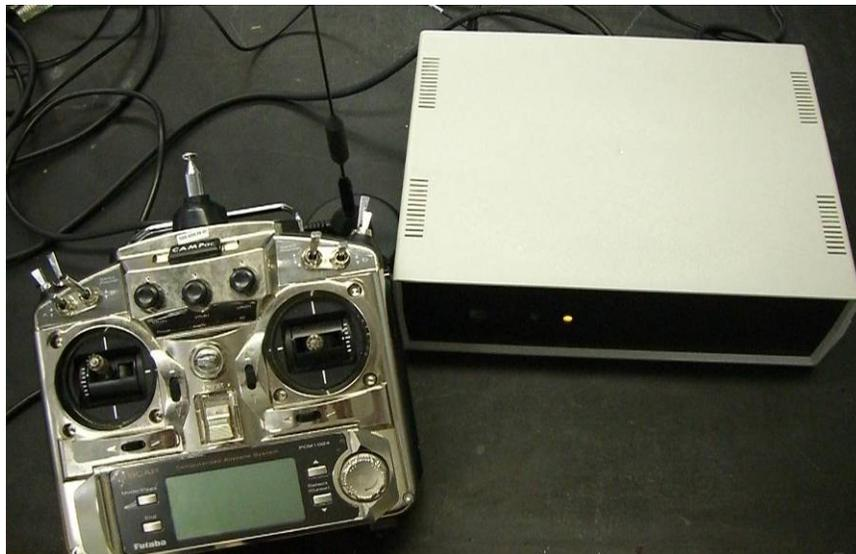
**Figure 6 – Piccolo Ground Station Hardware**
