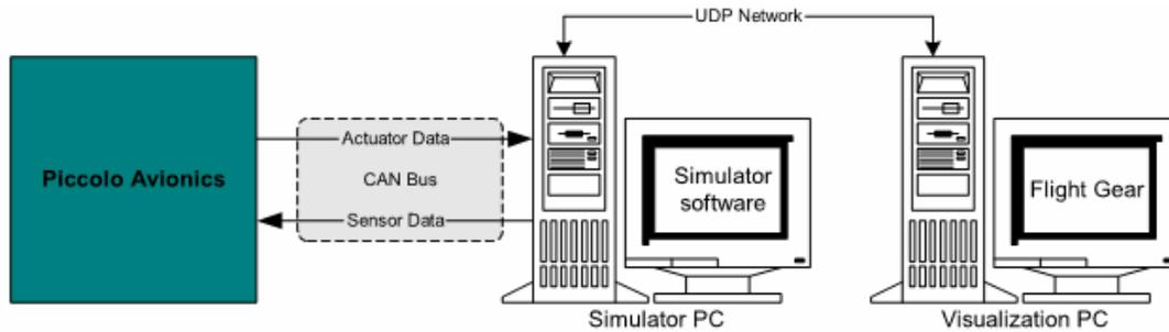
**Figure 11 – Hardware in the loop simulation<sup>3</sup>**
