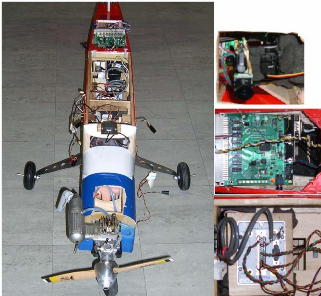
**Figure 2 – Southern Komfort UAV (left) and Camera (top right), Camera Control (middle right), Autopilot (bottom right) Subsystems**
