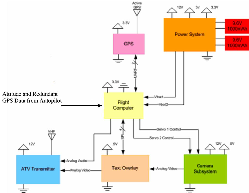
**Figure 8 – Camera payload block diagram**
