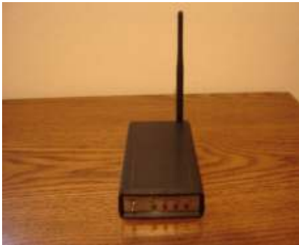
The 910 MHz Radio Modem is designed from Micro Hard.
