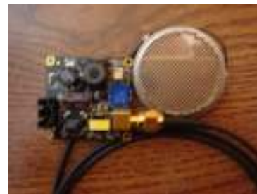
Ultrasonic sensor provides autonomous take-off and landing
