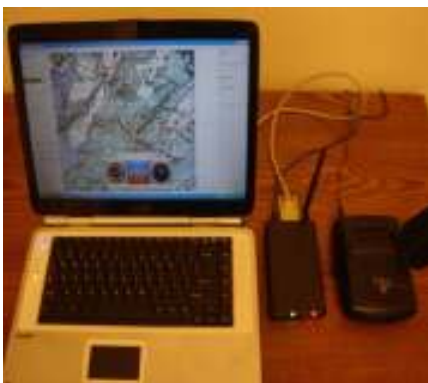
This is the Ground Station that included the MicroHard Radio Modem and the 2.4 GHz Camera receiver.
