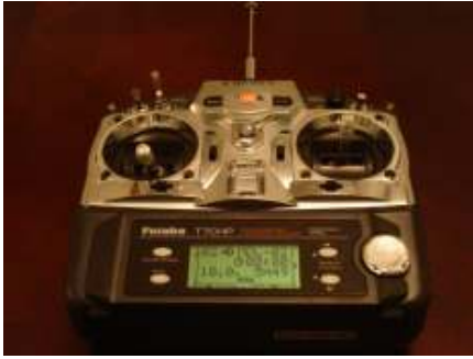
72 MHz PCM 7-Channels Transmitter for manual control
