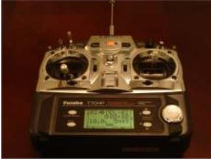
72 MHz PCM 7-Channels Transmitter for manual control
