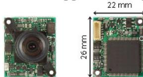
Figure 8: Wide-Angle Camera (front & back)
