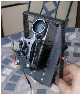
Figure 11: High-Resolution Camera on the pan-tilt-zoom-platform
