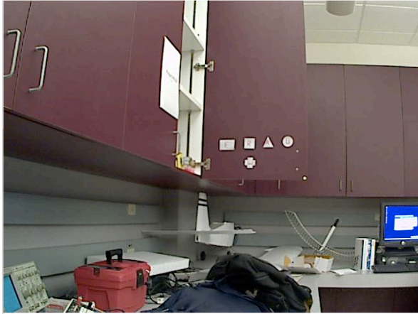
Figure 5. A lab test image using sub-scale targets. The targets and range are scaled to simulate 48 inch targets at 250 foot altitude. This test demonstrated that the camera and lens were a feasible solution for the mission requirements.
