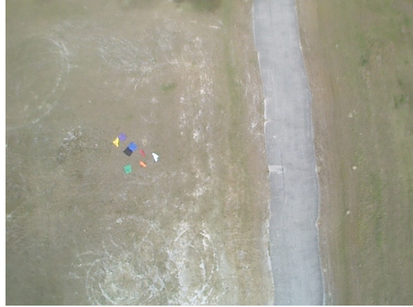
Figure 6. An example flight test image taken from 213 foot altitude. The 44-inch color targets are easily recognized, and the horizontal distortion due to vibration is acceptably low.
