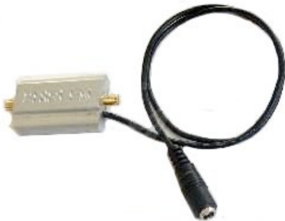
Figure 8. The 802.11b bidirectional amplifier. The amplifier is specified for 1000 mW output, and 16 dBi input gain.
