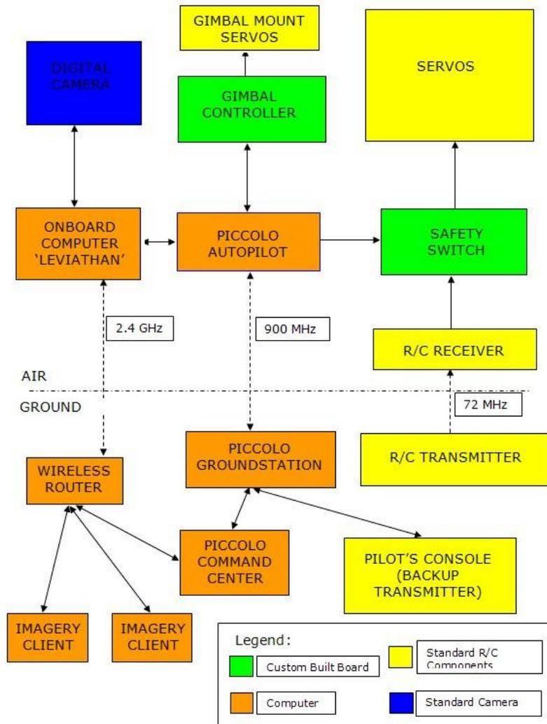
**Figure 1: Communications Diagram**
