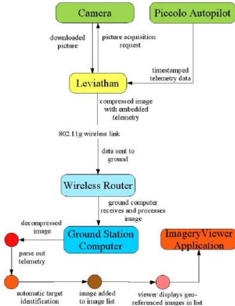
**Figure 3:** Imagery Communication Pipeline.
