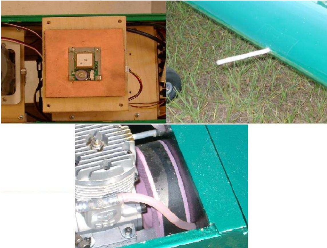
**Figure 2.** UWF UAS showing GPS module, wing mounted pitot tube and motor vibration damper.
