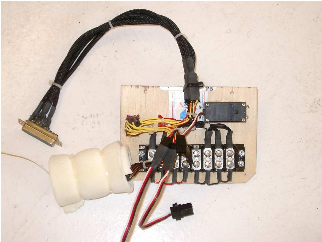
**Figure 6.** Electrical power distribution module.
