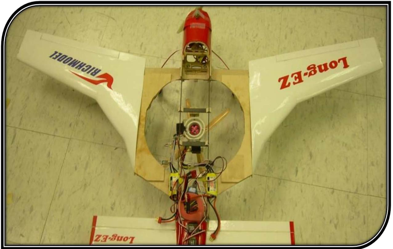
Figure 1: Long EZ, modified for VTOL capabilities
