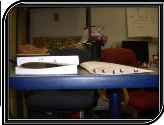
**Figure 4: Foam cutters and wing panel section**
