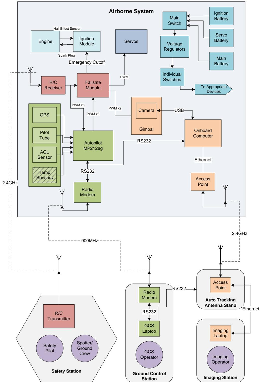
Figure 3.0.1: Overall System Block Diagram
