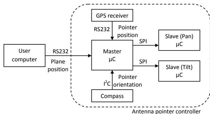
Figure 3.6.2: AATS Controller Block Diagram
