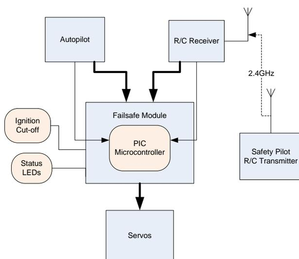
Figure 3.9.1: Failsafe Block Diagram
