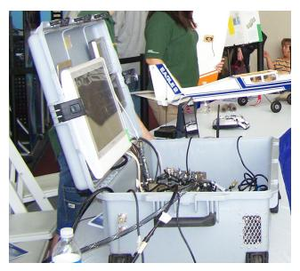
The Piccolo Plus in the plane relays information to a Ground Control Station (GCS) using a transmitter and receiver of an Ultra-High Frequency (UHF). This GCS in turn sends that information to a PC. The information is displayed on the interface of the GCS software. Subsequently, the internal pilots have the ability to adjust the plane as necessary from that information. Both the User Interface and the Pilot Console communicate with the plane through the GCS.
