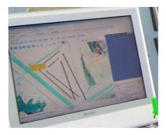
Internal pilots use the interface to control the plane autonomously. After being calibrated with the plane, the User Interface can send the plane orders, and the plane can send back information, such as global position, orientation, altitude, attitude, and airspeed. The internal pilots can create a preplanned path for the plane to follow autonomously during flight through the use of waypoints, which are exact locations on the map that the plane must fly to, one after the other.
