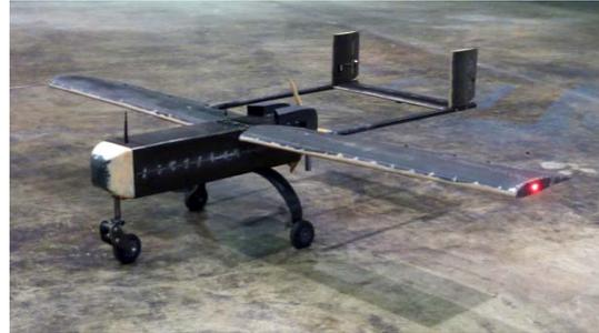
**Figure 4** — Xawk X-4 UAS Airframe Fully Assembled
