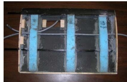
**Figure 11** — Vertical stabilizer showing foam ribs and spar rods.
