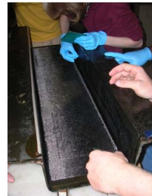
**Figure 9** — Fuselage shell formed in mold.
