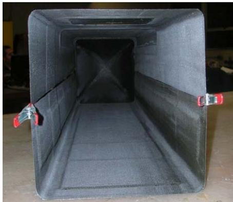
**Figure 10** — Two shells clamped together with nosecone.
