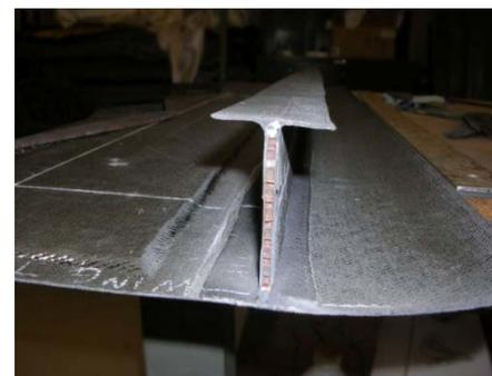
**Figure 12** — Custom ‘I’-beam spar used in Xawk X-4, shown bonded to lower skin.
