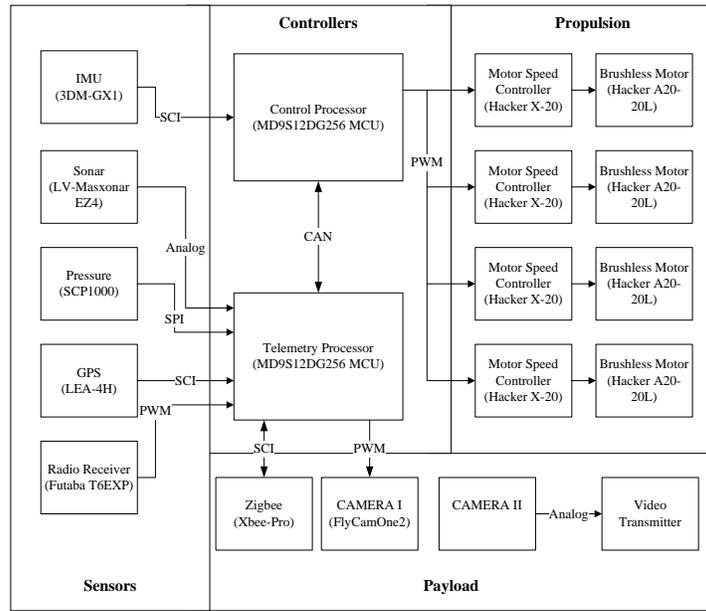
Figure 4. The Quadrotor Avionics
