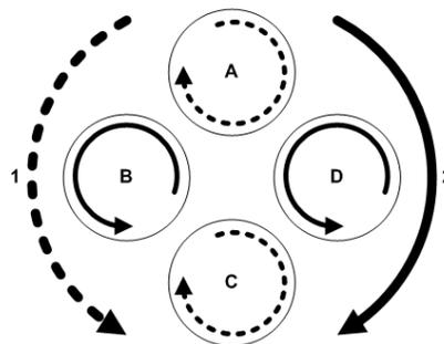
Figure 2. Quadrotor Reaction-Torque Schematic
