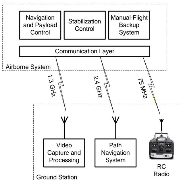
Figure 12. A High-Level View of Microraptor
