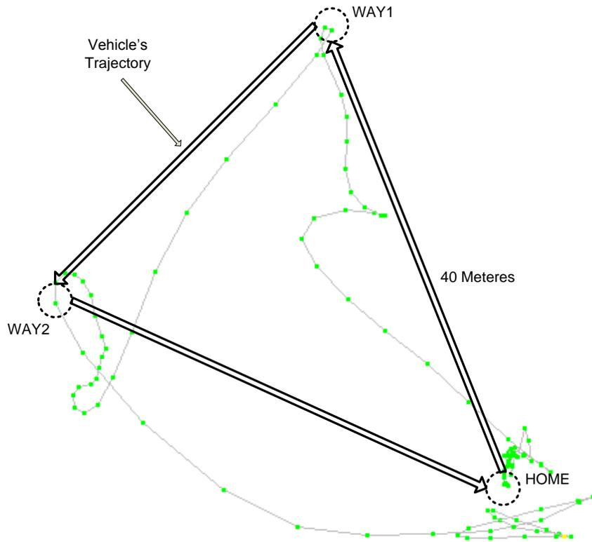
Figure 19. Position of Vehicle during the Waypoint Navigation
