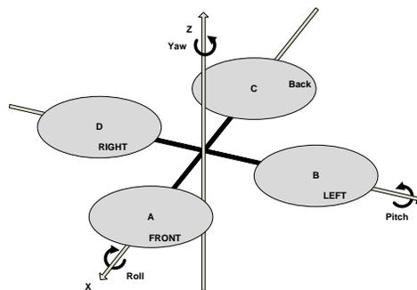
Figure 1. Rotational Motion of Quadrotor
