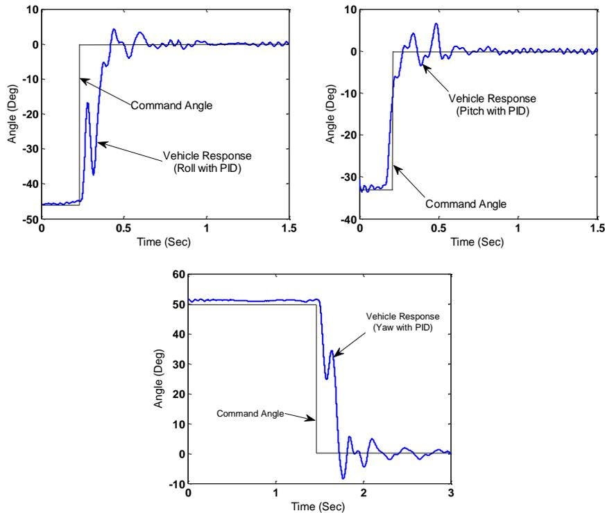
Figure 15. PID Control System Responses (roll, pitch and yaw)
