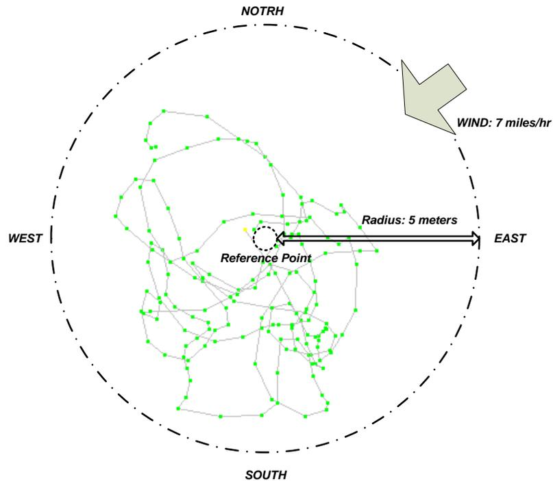
Figure 17. GPS Hold (Wind: 7Mph NE, Flight Time: 3 min, Altitude: 1.5 meters)
