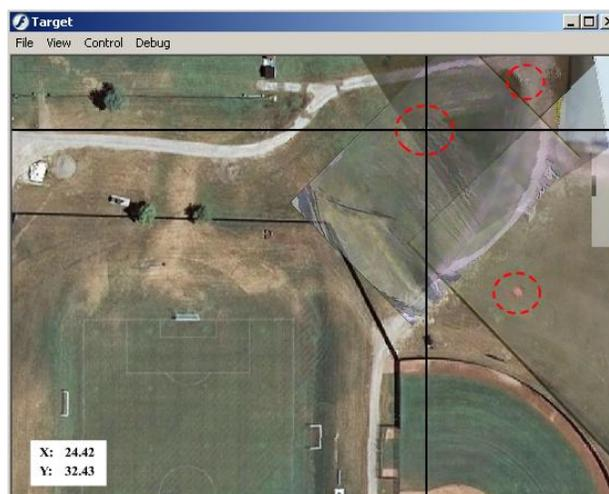
Figure 11. Macromedia Flash Program Still Image Processing GUI Showing 3 Targets
