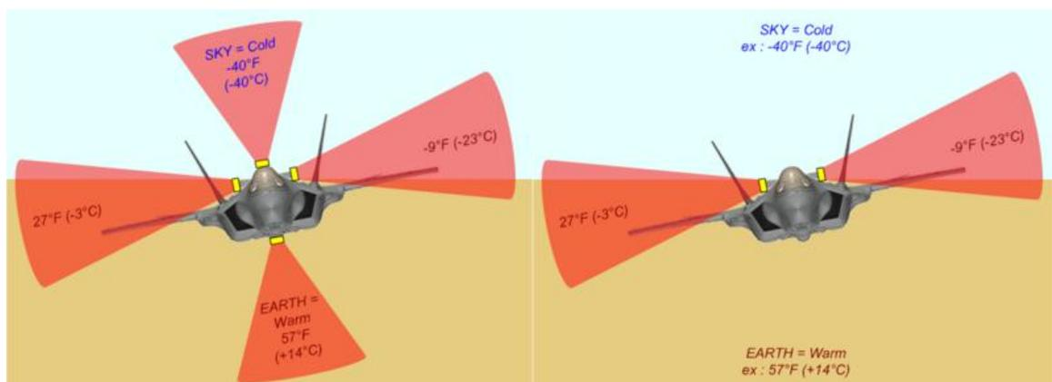
3 pairs of sensors are employed for the measurement of pitch and roll to enable deployment of autopilot systems. This 3 pair sensors array provides for better results as it eliminates the need for ground calibration which would otherwise be essential in the x-y array.
