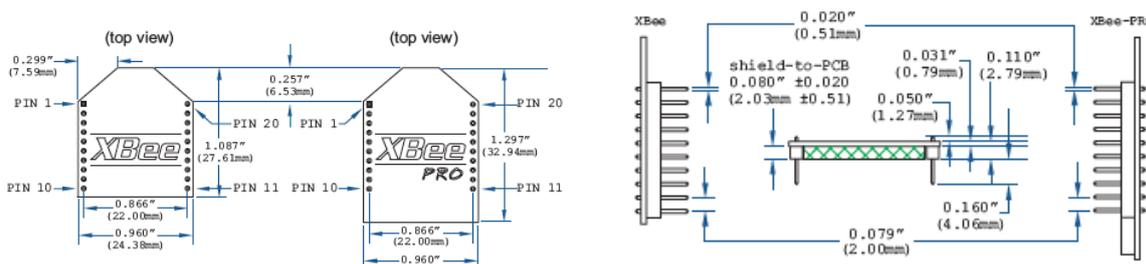
The XBee-PRO XSC OEM RF modules are extended-range 900 MHz devices providing end-point connectivity to devices. The modules are capable of deployment in point-to-point, peer-to-peer and point-to-multipoint networks. The versatility was the proving point for the choice of modems for telemetry.
