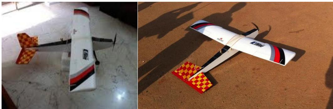
The team believed in building its own airframe, as it enhances the team's experience of flight construction and in the process has been able to analyse and eliminate faults in the airframe. The team experimented with a number of airframe designs, built about 3 to 4 fuselages and sets of wings before freezing and selecting the current form and function.
