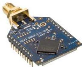
The team is using a 900 MHz XBee-PRO XSC pro modems in the telemetry unit. Ease of use and efficiency were the primary factors in choosing the XBee-PRO XSC. The XBee-PRO XSC are capable of Outdoor RF line-of-sight range up to 15 miles (24 km) with high gain antenna and Outdoor RF line-of-sight range up to 6 miles (9.6 km) with dipole antenna.
