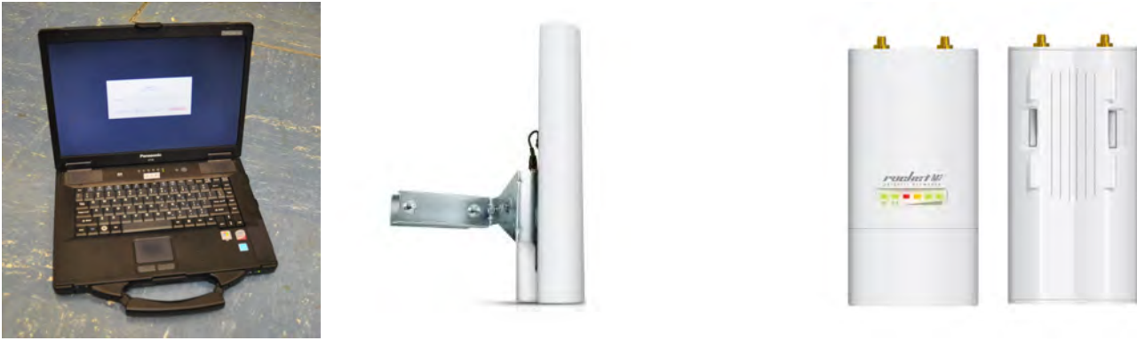
Figure 16: GCS laptop, Rocket M Wireless AP, Airmax Sector Antenna
