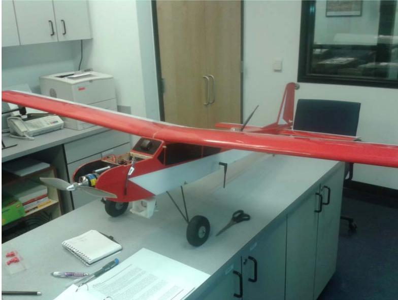
Several modifications were made to the stock airframe, primarily strengthening the landing gear and wing struts, but also constructing frames within the fuselage to mount electronics. Because of the large size of the flight batteries, mounting points were constructed on the underside of each wing, freeing space inside the fuselage for other systems.
