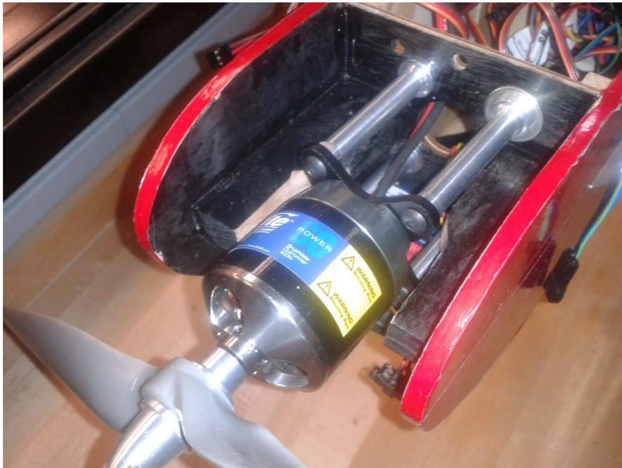
Using a 15/8 propeller lets this plane achieve a few things. The propeller being used is from American Propeller Company (APC) which has a much more aggressive pitch towards the hub
