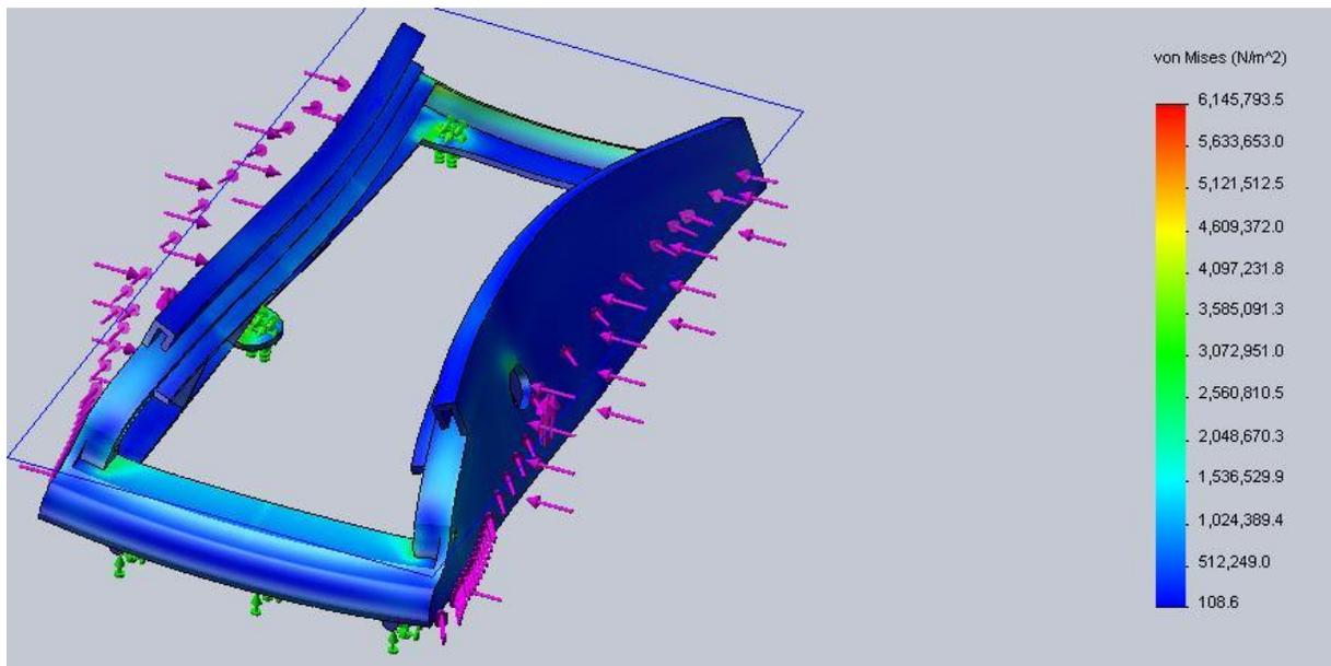
Figure 7: Isometric Von-Mises Stress Graph
