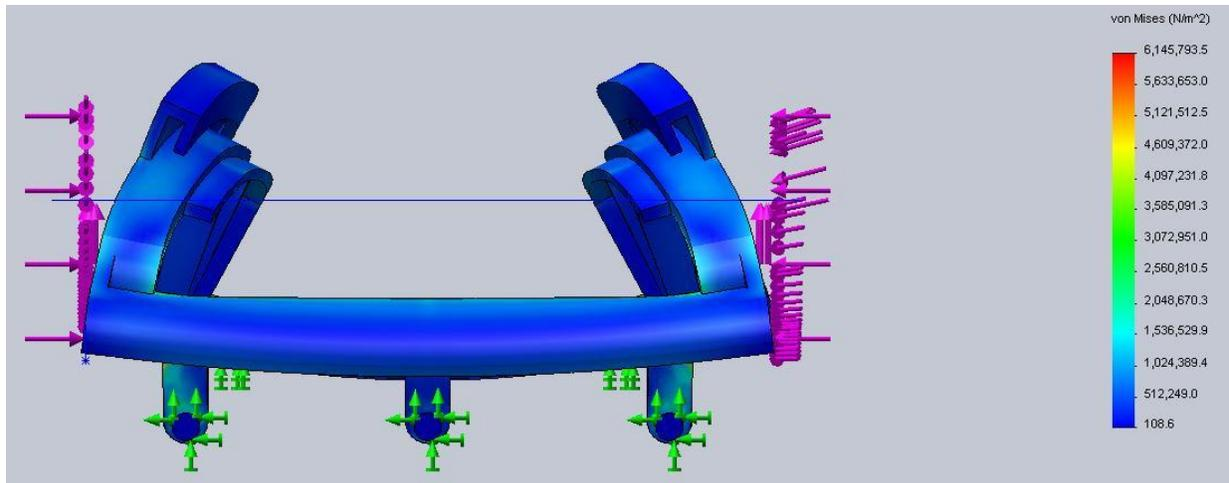
Figure 8: Front Von-Mises Stress Graph
