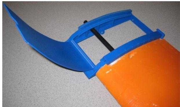
**Figure 4: Hatch and wing attachment - open**
