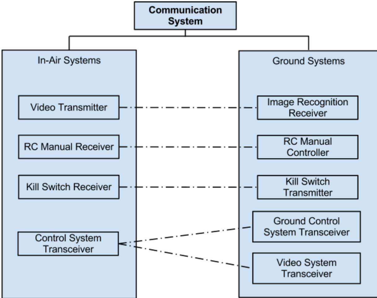
Figure 6: Communication systems diagram
