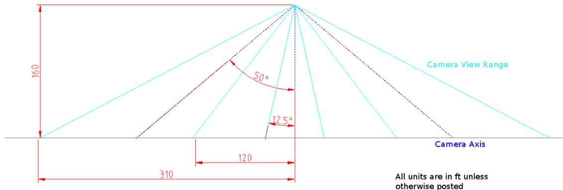
Figure 5: Vision system parameters
