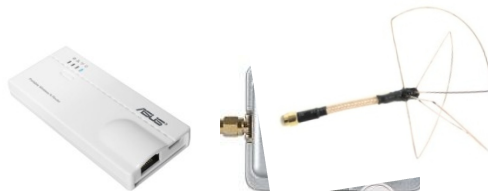
Figure 12: On-board Router, Amp and antenna
