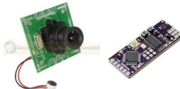
**Figure 8: CMOS Camera/Minim OSD**
