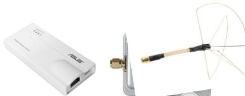
**Figure 12: On-board Router, Amp and antenna**
