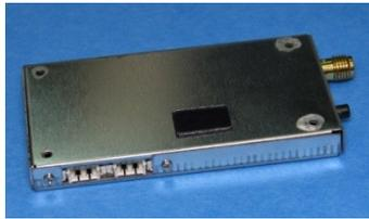
**Figure 11: 1.3 GHz Transmitter**
