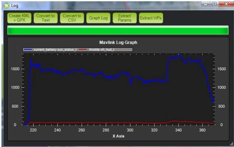
**Figure 3: Battery Current/Throttle Analysis**
