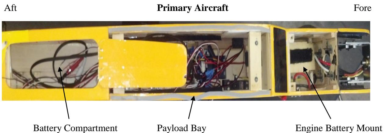
The primary aircraft being used is a 2011 model Senior Telemaster airframe that has been modified to hold an autopilot and camera mount in order to complete the assigned tasks. The plane has a wingspan of 95", length of 60" and an empty weight of 12.9 lbs. It is propelled by a 1.20 Rimfire electric motor which is powered by a 6S 5000mAh motor pack. The propeller is a 16x8 and is manufactured by Master Airscrew.
