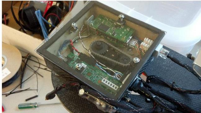
The imagery data is sent by a 5.8 GHz Wi-Fi modem capable of two way communication. This provides long range transmission of data from the aircraft to the receiver. Live video is sent real time to the payload operator.
