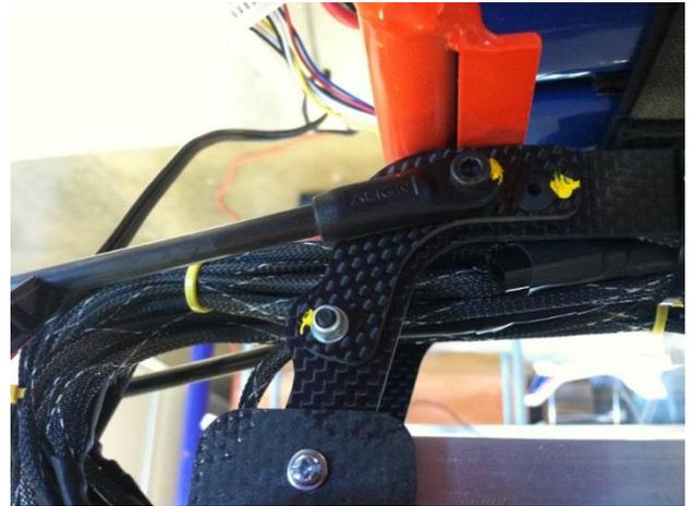
Torque Paint, Wire Sleeves, Zip Ties and High Visibility Paint
