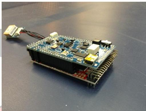
Picture of the Autopilot Board without the telemetry attached
