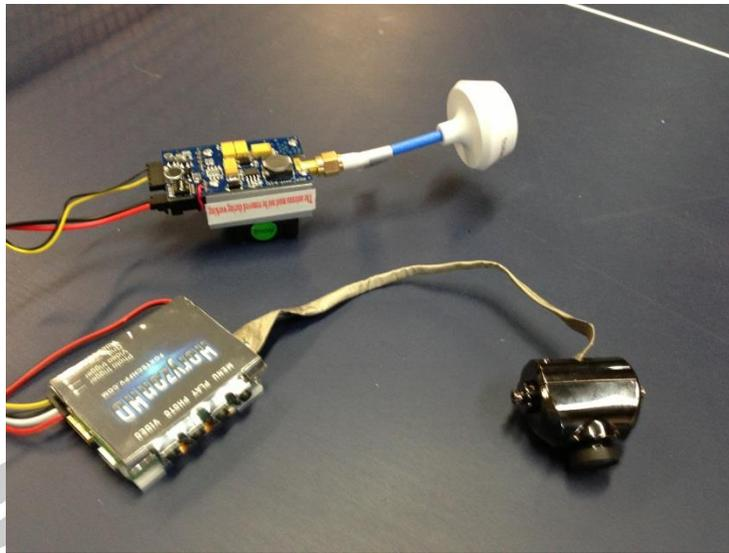
This is an image of the camera system and the 5.8GHz transmitter
