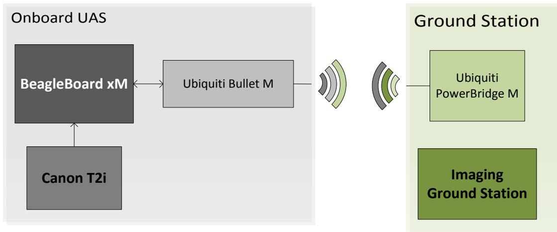
*Figure 5: Imaging system block diagram*
