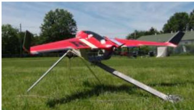
*Figure 2: Launcher with UAS*
