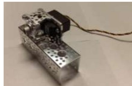
*Figure 4: Camera stabilization gimbal*
