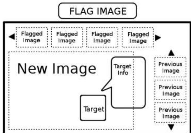
*Figure 8: Imaging ground station software schematic*
