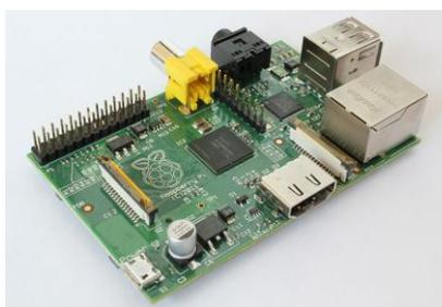
Figure 6: The Raspberry Pi single-board computer
