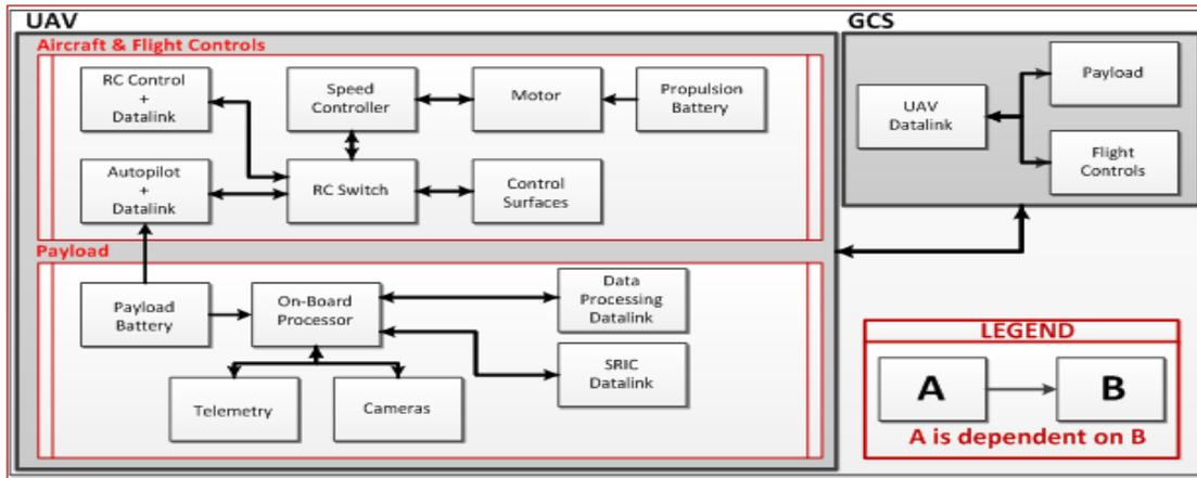
**Figure 1** UAS Design Breakdown and Dependencies
