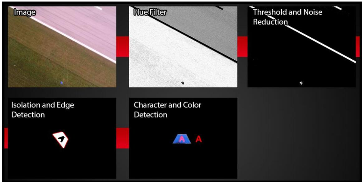
Figure 7 IMAGE RECOGNITION PIPELINE
