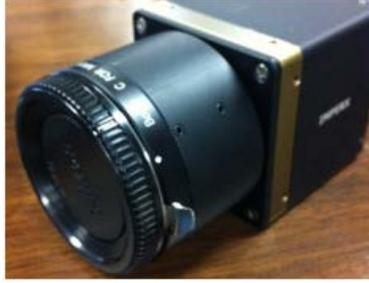
**Figure 2 – Imperx BOBCAT IGV-B4820 camera**
