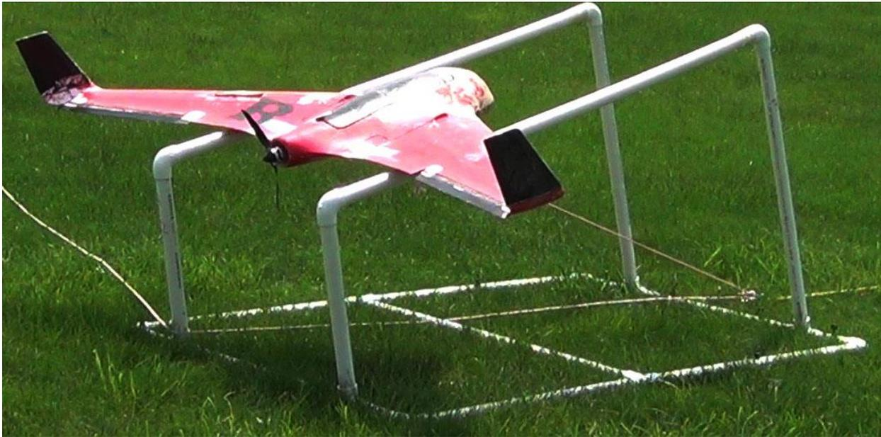
The launcher is relatively easy to transport and set up, as it is simply a number of pieces of PVC and a ground stake. Setup can be handled by the team in a matter of minutes with a few simple tools.
