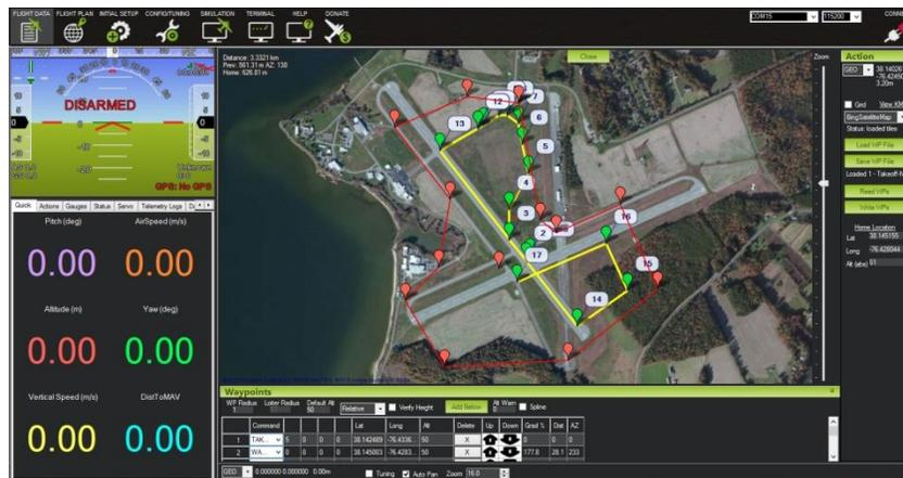
**Figure 2.5-1: Picture of Mission Planner Interface with a Flight Mission
