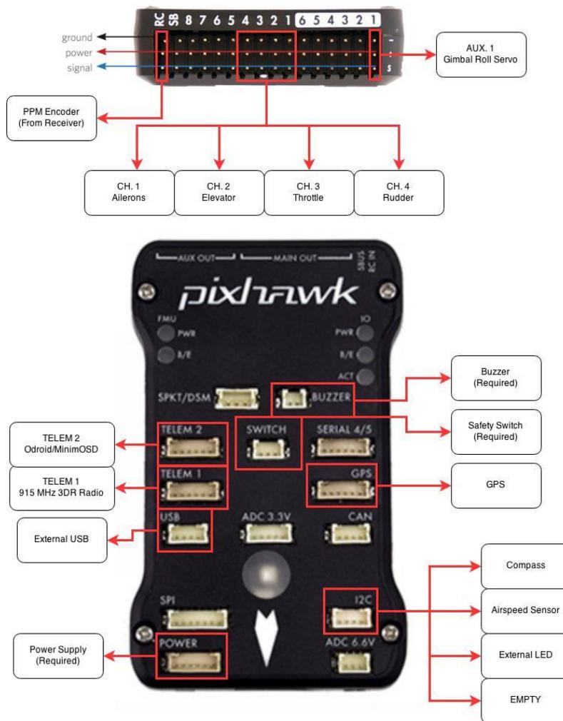
FIGURE 7: PIXHAWK<sup>®</sup> WIRING DIAGRAM
