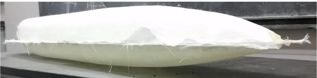
**FIGURE 1: FIBERGLASS FUSELAGE DURING CONSTRUCTION**
