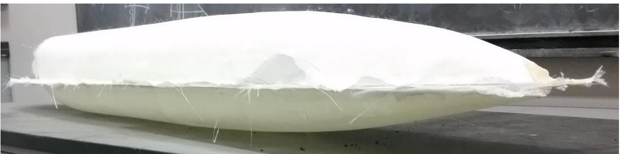
FIGURE 1: FIBERGLASS FUSELAGE DURING CONSTRUCTION
