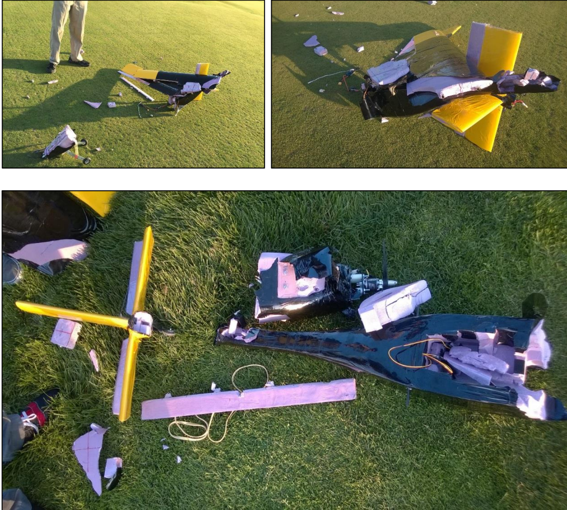
Figure 7, 8, & 9: Prototype 2 (Genie) After Experiencing Error in Wing Fabrication
