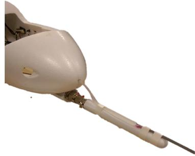
**FIGURE 4 - UBIQUITI BULLET AND PITOT TUBE MOUNT**
