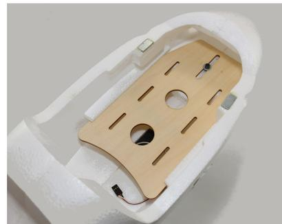
**FIGURE 2 - ADJUSTABLE FUSELAGE TRAY**
