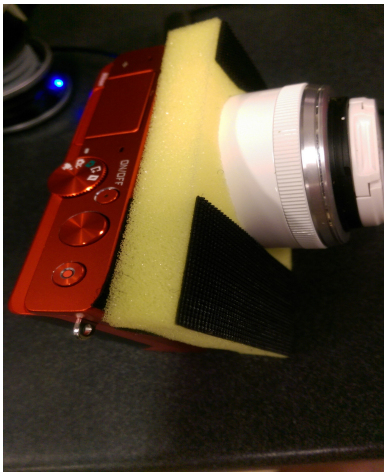
FIGURE 3 - CAMERA SHOCK-ABSORBING SPONGE
