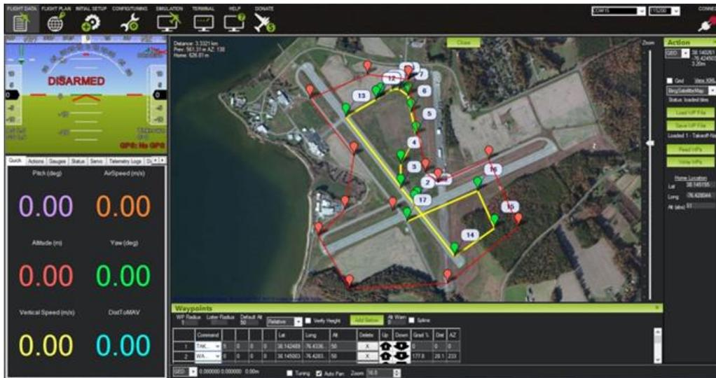
**Figure 2.5-1: Picture of Mission Planner Interface with a Flight Mission (Red is the Boundary for the No Fly Zone)**
