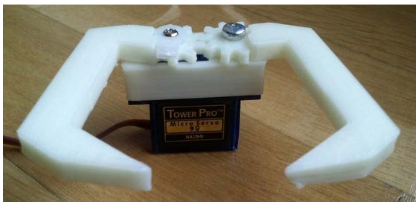
Figure 6: Representation of the payload drop mechanism
