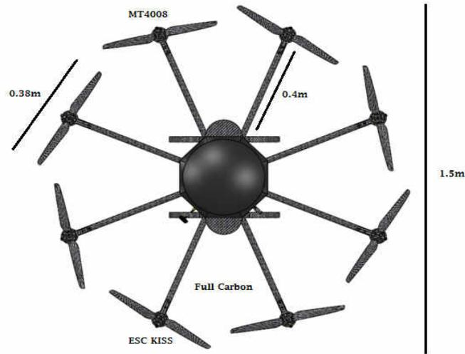
Figure 1. UAV physical model (from CAD plan)
