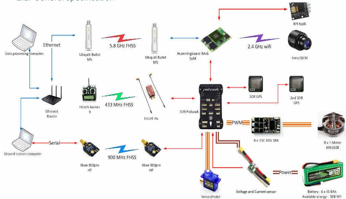
Figure 3. Complete system wiring schematic
