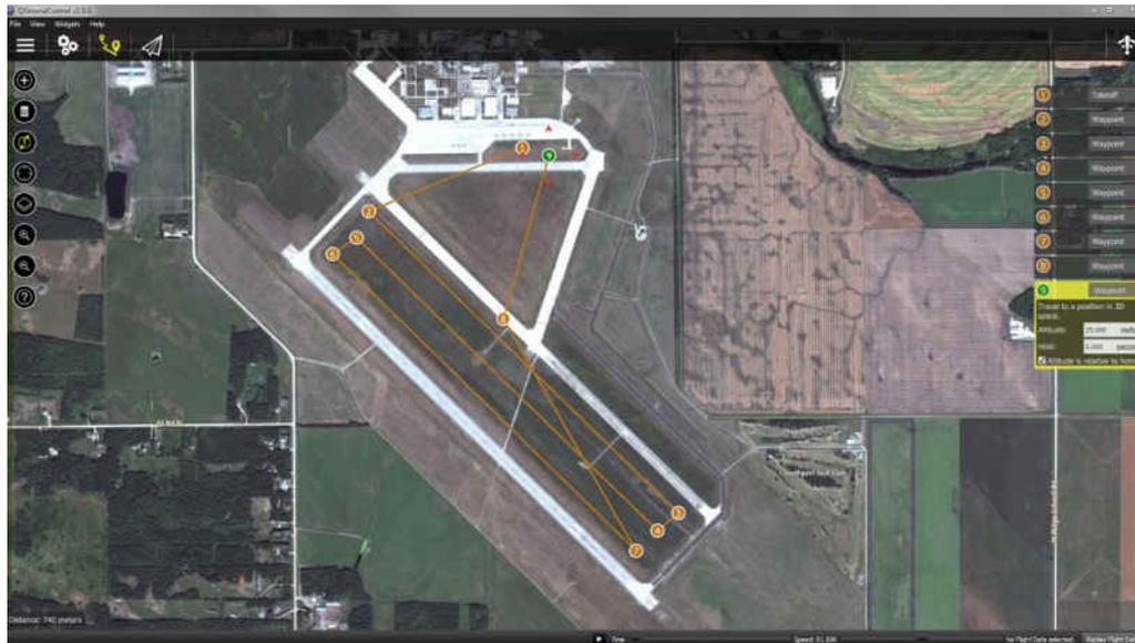
Figure 7. Mission example on QgroundControl
