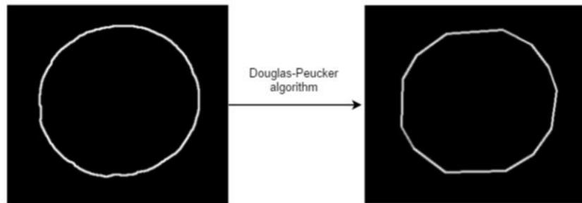
**FIGURE 7 - SHAPE DETERMINATION**
